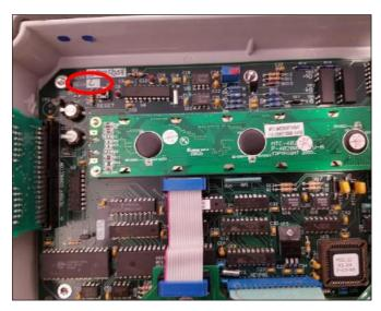
Now both memory cards have the same settings saved on them. Before powering up to operate, be sure the original "old" memory card is in the "old" controller and the "new" memory card is in the "new" controller.
