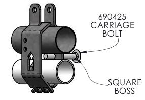
INSERT A 690425 CARRIAGE BOLT INTO THE SQUARE HOLE ON THE BACK CLAMP, BETWEEN THE CONDUIT AND THE WATER PIPE, THROUGH THE SQUARE HOLE ON THE FRONT CLAMP
