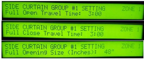
2. Keeping the curtain in calibration can avoid out of position alarms. Setting a once a day Resync time will help by ensuring a full open or full close calibration (whichever is closest) at the time of day set.
