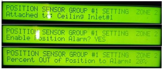
ii. **Ceiling Inlet Settings** (Press hotkey next to toggle switch then arrow "Down") – Does the full opening size match what is measured with a tape measure? Do
