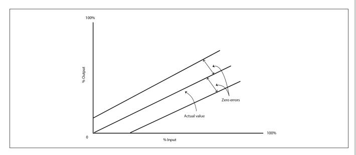
To correct the problem, the output of the sensor must be calibrated to be linear and represent the measure.
