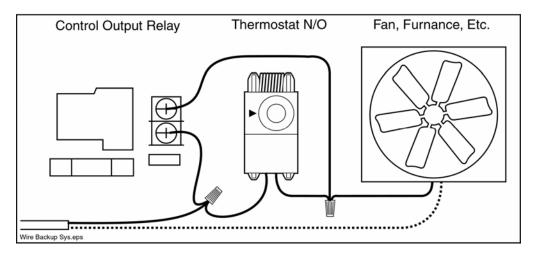
Thermostats should be installed to backup heaters, fans and inlets. Natural ventilation buildings need curtain drops. Thermostats can be wired to the devices they will operate, and in parallel with the GainTRAC as shown above.
