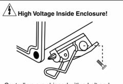
Controllers are shipped with a bolt and nut to hold the quick release latch closed. You can remove the bolt and nut during the installation process. You must replace these after installation to protect against accidental exposure to the high voltage inside the enclosure.
