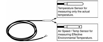
Connect sensors to the input/output board as shown below making sure to ground the shielding as well as the black wire.
