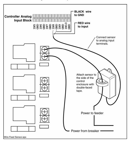
The best use for a single feed sensor is monitoring your silo auger motor. This provides a clear indication of all feed entering the building and it provides an alarm when the feed silo is empty.
