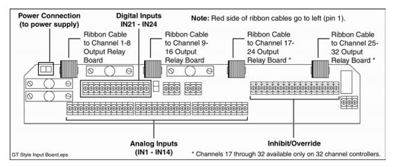
Some inputs have a 12V output that is required by certain sensors. Analog terminals 1 through 4 and all digital inputs have the 12V output available.
