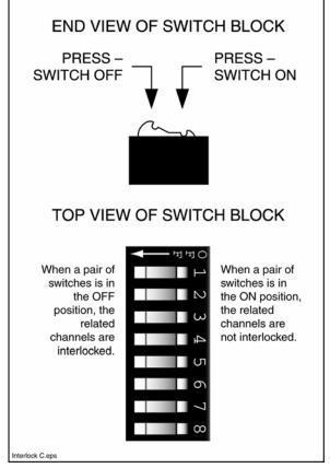
interlocked. When ON, the channels are not interlocked.
