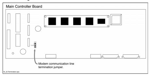
If the GainTRAC **is not** at the terminal end of a group of GainTRAC controllers and a communications station, the GainTRAC modem communications line needs to be un-terminated.
