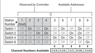
16 and 32 channel GainTRAC and Ventra PLUS controllers use the expansion station address as part of the channel number. Example; an Expansion station with an address of 5 would contain channels 51 and 52.
