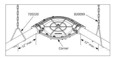
1. Add support on each side of the corners, as shown above. Corners should be a minimum of 24" (60.96cm) apart.
