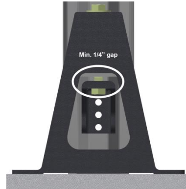
Figure 5: Leave 1/4" (+/- 1/8") gap between C-channel and bracket.
