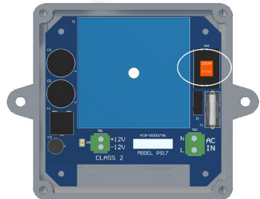
Figure 9: Red toggle switch changes from 115V to 230V.
