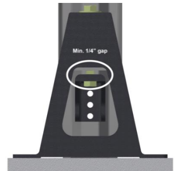
Figure 5: Leave \frac{1}{4} " (+/- 1/8") gap between C-channel and bracket.
