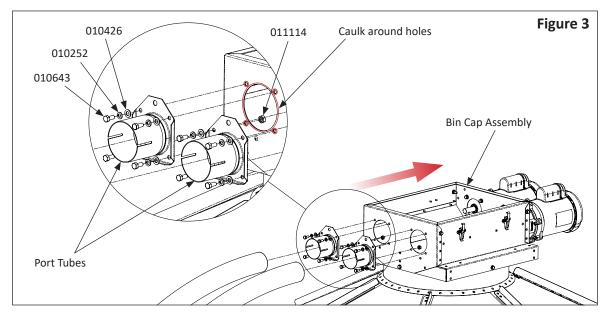
Step 5: Caulk around holes then install Weatherhood to the Bin Cap Assembly over Gearboxes/Motors using hardware supplied in 506290 Twin Fill System Hardware Bag: (4) 501442 bolts and (4) 501441 nuts, as shown in Figure 4.
