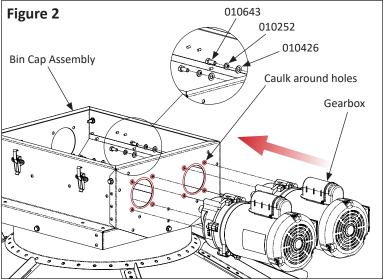
Step 4: Caulk around holes and then install Port Tubes to the Bin Cap Assembly using hardware from the Port Tube Hardware Bag, as supplied with the Port Tube and Driver Assembly: (4) 010643 bolts, (4) 010426 washers, (4) 010252 lock washers, and (4) 011114 nuts per Port Tube Assembly, as shown in Figure 3. NOTE: If installing 740 Port Tubes, mark and drill new holes for the bolt locations.
