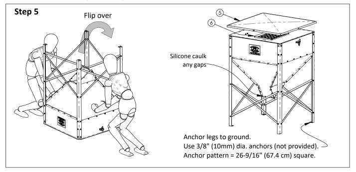
The 500820 transfer hopper is not intended for use in outdoor feed storage. The hopper should only be used to transfer feed with an auger connected to the bottom outlet. Connect a VAL-CO slide valve with hardware provided with valve. PVC auger tubes need to be supported every 4 ft with chain or structure. Customer is responsible for auger tube support. Reference Flexible or Rigid Auger manuals for more information.
